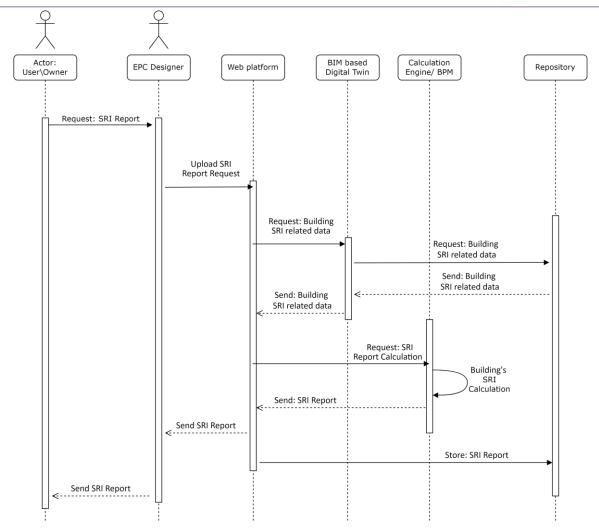
Figure 27. UC1.3 Sequence Diagram
