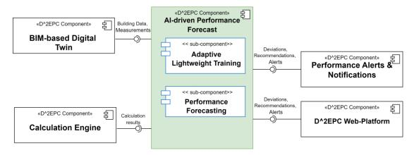
Figure 16. Al-driven Performance Forecasts Functional Diagram
