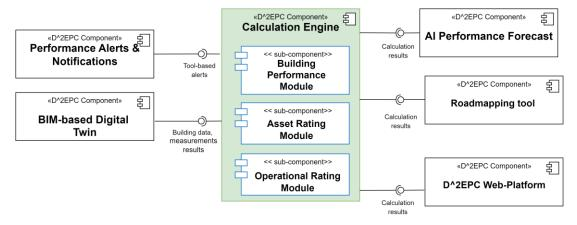
Figure 14. Calculation Engine Functional Diagram
