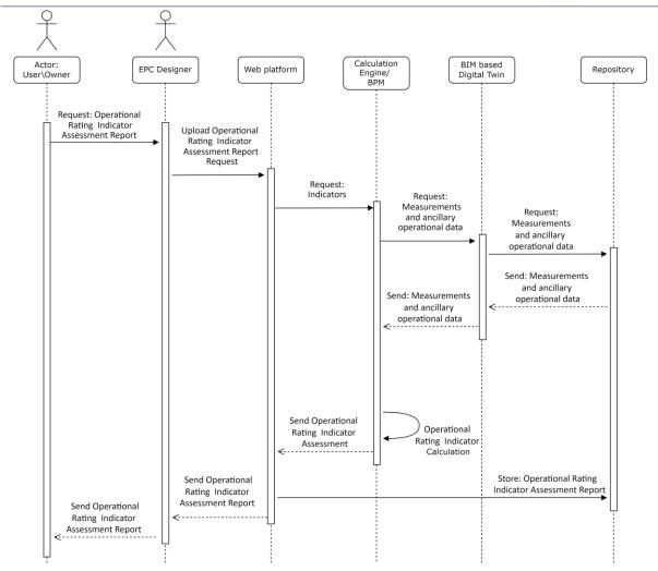
Figure 33. UC2.3 Sequence Diagram.
