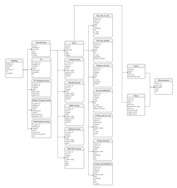
Figure 23. D^2EPC data model including basic elements information
