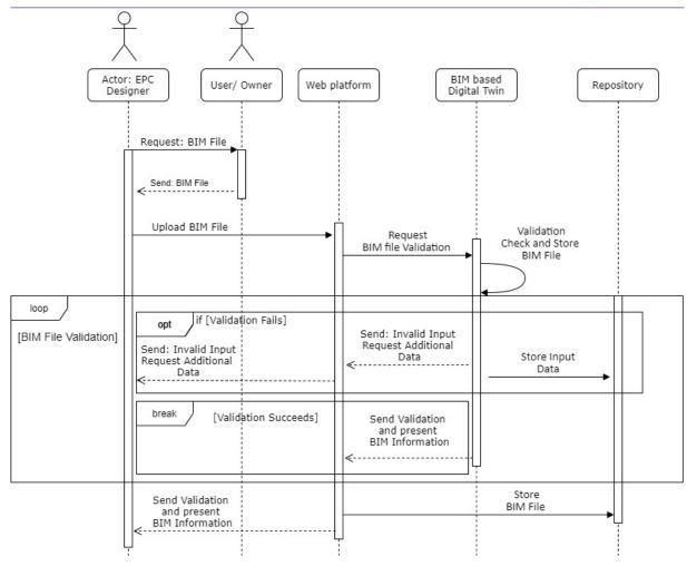
Figure 25. UC1.1 Sequence Diagram
