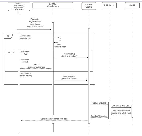
Figure 39. UC4.1 Sequence Diagram.
