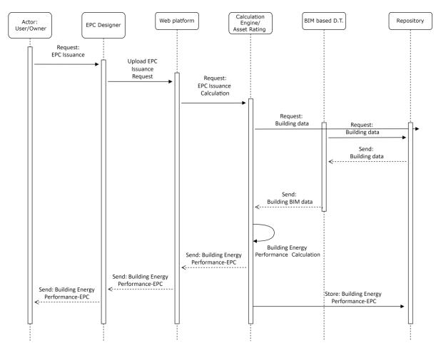
Figure 26. UC1.2 Sequence Diagram.
