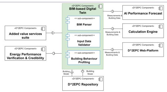
Figure 13. Building Digital Twin Functional Diagram
