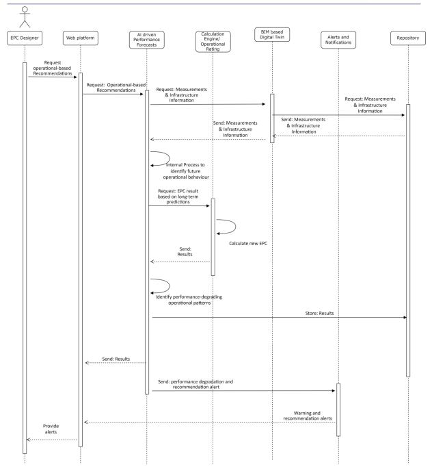
Figure 34. UC2.4 Sequence Diagram
