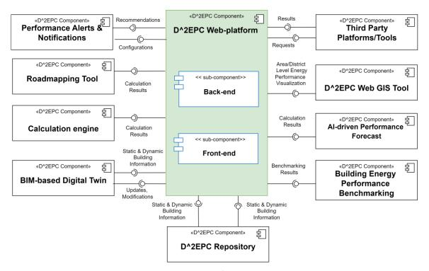
Figure 20. D^2EPC Web Platform Functional Diagram
