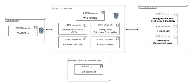
Figure 24. D^2EPC High-Level Deployment Diagram
