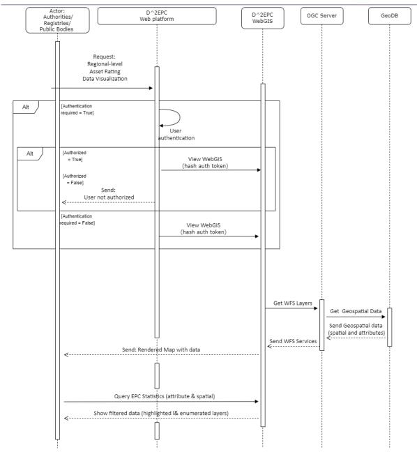
Figure 40. UC4.2 Sequence Diagram.
