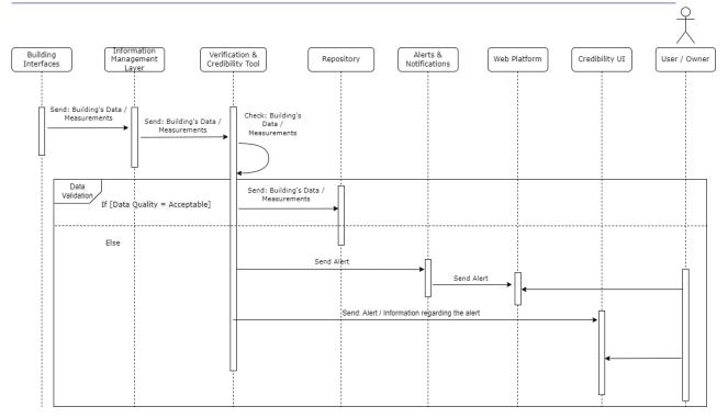
Figure 31. UC2.1 Sequence Diagram.
