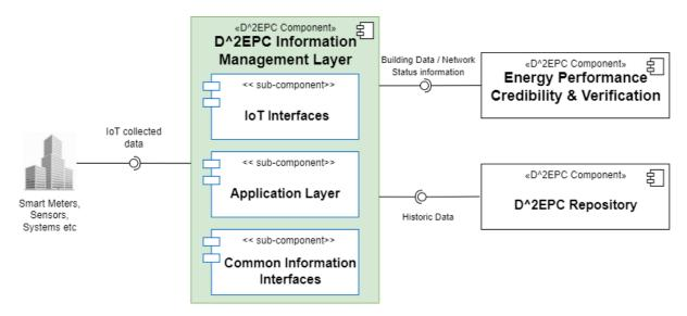
Figure 11. D^2EPC Information Management Layer Functional Diagram
