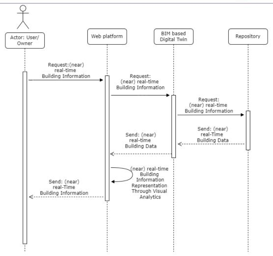
Figure 36. UC3.1 Sequence Diagram.
