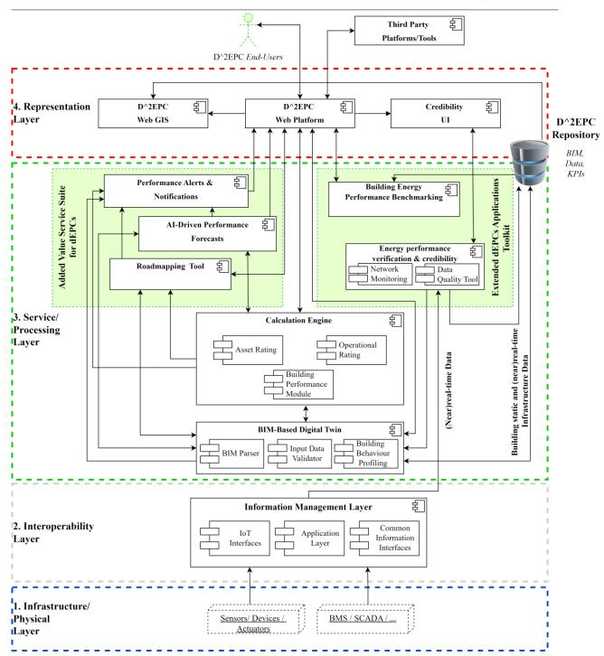
Figure 9. D^2EPC Layered Conceptual Architecture
